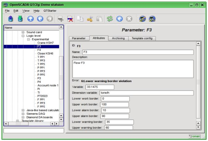
Fig. 4.51. The "Attributes" tab of the parameter of the controller of subsystem "Data acquisition".
