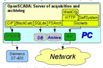
Fig. 3.1. Simple server connection.
