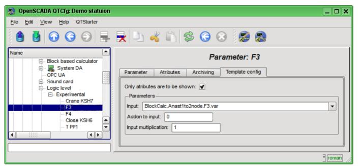
Fig. 4.5n. The "Template config" tab of the parameter of the controller of subsystem "Data acquisition".
